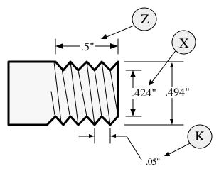
For this part the X zero is at the center of the part. The Z zero is at the face of the part.
