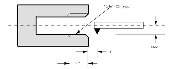
In the above example we will be cutting a 15/16-20 internal thread. (written in radius mode, G73):
