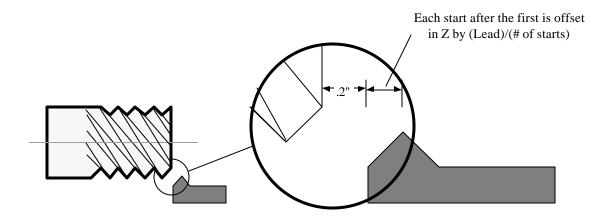
**Value of Z**: The starting position of Z is offset for each start by (pitch)/(number of starts). IE. if we have a three start thread the first start is at the normal .2" from the face of the material. The second start is offset by .2" + (.15/3) = .25. The third start is offset by .25 + (.15/3) = .3
