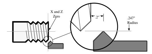
The locations shown above are given in radiuses. The starting location in X is the major diameter, less the amount of the first pass. In this case the major diameter is .494", half of this is .247". Less .01 to be taken for the first pass: .237
