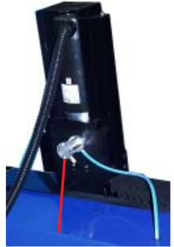
from the control and make sure there are no cracks that will allow coolant to enter the cable. If the outside jacket is degrading it is possible to replace it in the field. Contact technical support for the jackets and tools required to remove the pins for the cable end. (10 minutes to replace the cable jacket, each.) (Monthly)
