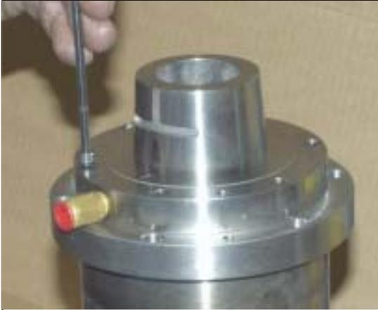
Turn the assembly over and remove the screws from the collar on the front.
