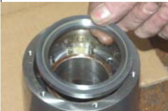
Under the back bearing there is a ring that goes over a set of springs. Make sure you really don't loose this! Make note as to how it comes out. It must go back the same way!!!
