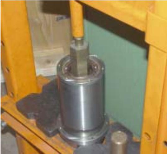
With an arbor press, carefully press the spindle out through the front of the cartridge. Don't let the spindle drop out and hit you on the foot. It is heavy.
