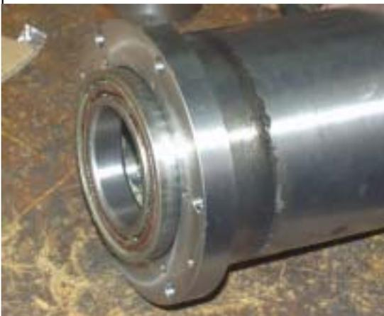
Here is the bearing in the front being removed by tapping from the rear with a brass bar.
