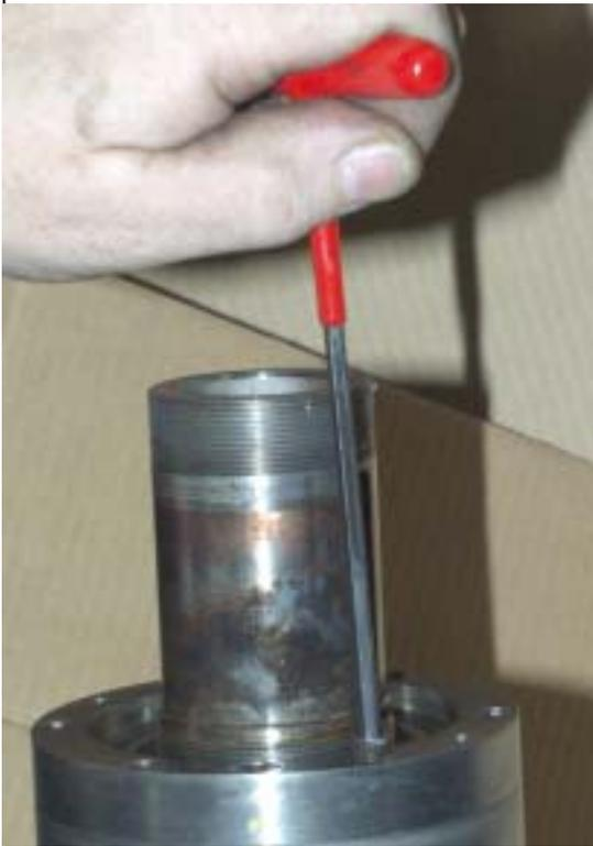
Remove the screws from the collar, don't loose these either.
