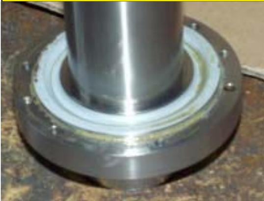
Check the front seal on the spindle. It is fragile, take care not to dent or damage.
