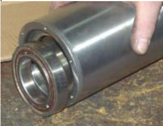
Here is the bearing after it has been removed from the housing
