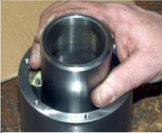
Pull the spindle sleeve out.
