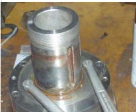
**Remove the threaded ring holding** the spindle core in the bearings. This collar threads off right handed. A spanner wrench is strongly suggested. Here we had to hold the other end of the spindle in a vise.
