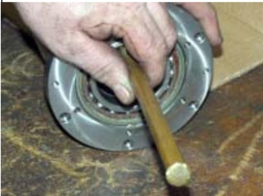
The bearings must now be removed from the housing. With a brass rod tap the bearing out the back first. Be carefull, there are some springs and a collar. Look at the next few steps first before you do them.
