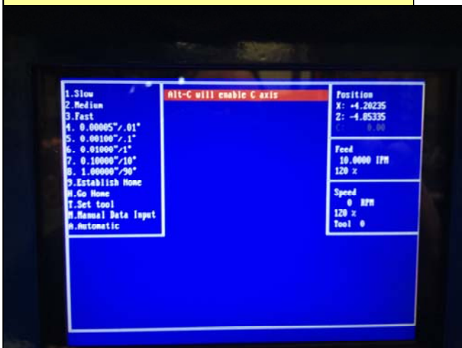
1: Start machine, get to the Jog mode and Home the machine normally
