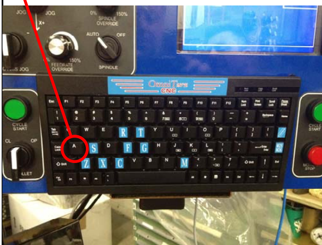
2: After homing press A for Automatic and select any program
