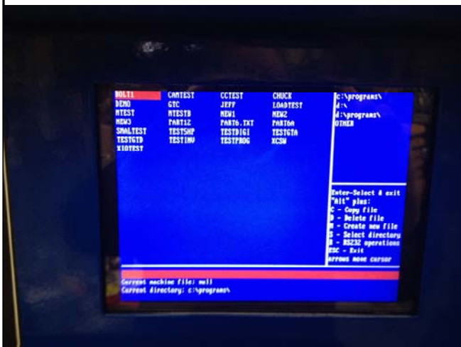
2: After homing press A for Automatic and select any program
