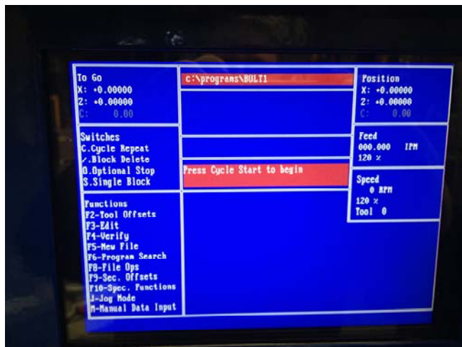
4: Press F3 to go to the editor Then press ESC key to not create a new file
