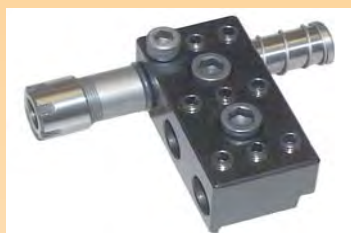
The tap holder will fit in all of the tooling bars with a 5/8" bore. Uses ER-16 collets
