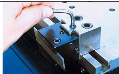
THE LOCKING WEDGE IS DRIVEN BY A SCREW FROM ABOVE
